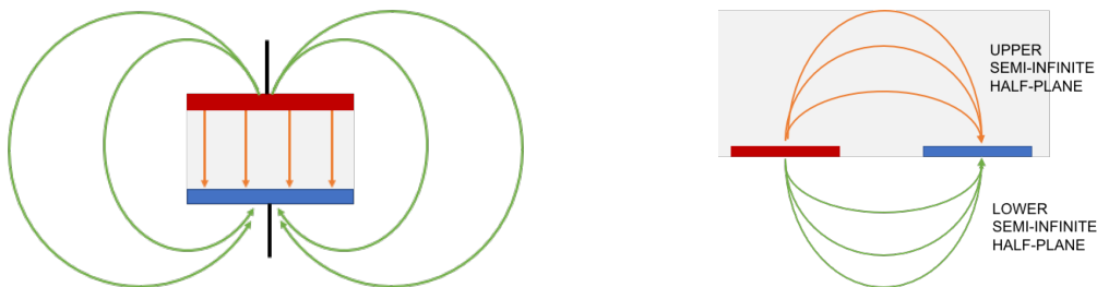
Figure 3.8: Parallel plate electrodes and coplanar electrodes
