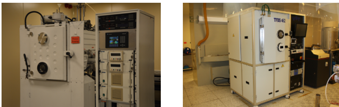
Figure 3.15: The VACOTEC Dual E-gun evaporation system (left) and the VST - TFDS 462 (right) in Winfab at UCLouvain, both used for the deposition of aluminium electrodes (thickness 1 \mu\text{m} ) on nitrocellulose [206]
