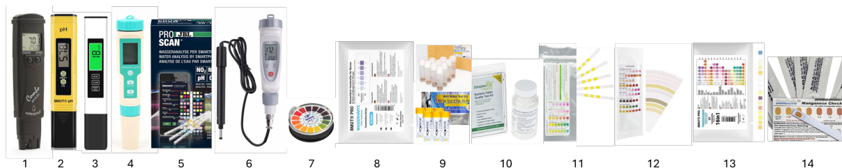
Figure 5.2: Ranking of user-friendliness of the different sensors 1. HI98130 pH/EC/TDS; 2. BMUT pH; 3. BMUT EC/TDS; 4. Unbranded PH/EC/TDS/Salt/S.G./ORP; 5. JBL PRO SCAN test strip; 6. DO sensor; 7. Universal pH paper; 8. BMUT Hardness test strip; 9. Medasa and Aquavial test bottles; 10. SimplexHealth test bottle; 11. SimplexHealth test strip; 12. Smardy Blue test strip; 13. BMUT 16 in 1; 14. Manganese test strip
